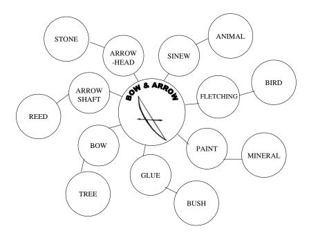
Figure 2.2 Elements of a bow and arrow
